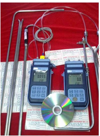
The BI 211P.0 and BI 211P.2 BI 213P.0 and BI 213P.2 are portable micro-manometers using Pitot tubes and a large LCD display. They are used to perform measurements in the fields of air conditioning, heating and ventilation. They measure differential the pressure detected by a Pitot connected instrument inputs acquiring the wind speed and flow rate inside pipelines and vents. They also measure the temperature using a type K thermocouple sensor.
