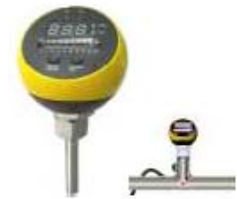
MODEL NO : BI0004 DIGITAL FLOW SWITCH DISPLAY : VELOCITY SMART FLOW SENSOR FLOW + TEMPRATURE SENSOR COMPACT TYPE FOR ADAPTOR SENSING MEDIUM : AIR, LIQUID LIQUID FLOW RANGE : 3....300CM/S GAS FLOW RANGE : 200...3000CM/S TEMPRATURE RANGE : 25....80deg.C OUTPUT SWITCHING (NPN/PNP NO/NC) ANALOG (4 – 20Ma) RELAY DISPLAY : LED
