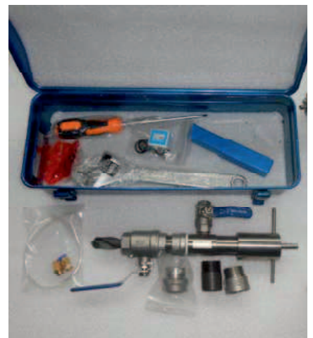
Hot tapping driller
